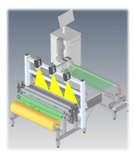
100% camera control is an important procedure when the application for woven mesh does not allow any flaws and documentation are needed. The system consists of high resolution cameras, which continuously take images of the mesh. As the mesh is exposed to the cameras, it identifies and tracks all defects, including large openings, small openings, broken wires, physical damage and more.
