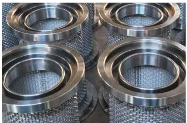
Produktion Filterelemente / Fabrication of filter elements
